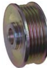
136452 Pulley Servicing: 5233449, 5233660, 5233949, 5233973, 5234029, 5234260 O.D. 63.10, W. 28.40, Grooves 5, Bore 17.00
