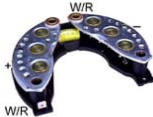
131573 Rectifier Replacing: UBB238 Diode Amp. 35, O.D. 115.00, I.D. 46.00 w/ Capacitor.
