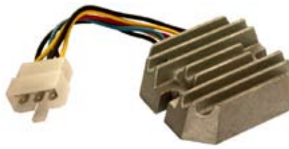
234414 Regulator/Rectifier Replacing: AM126304 14 V. Terminals: B+(red w/ blue), -(black), AC(yellow), L(brown), AC(yellow).
