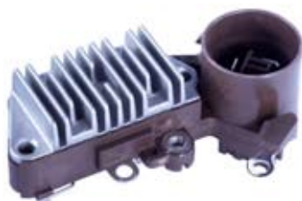
131459 Regulator Replacing: UCB412 14 V., V. setting 14.4, Terminal type S-IG-L Repair Circuit: Cargo 133235. L-Terminal drives the choke.
