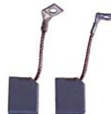
JX222 Brush Set Replacing: 74996331 12 V., L. 20.50, Th. 6.00, H. 16.00
