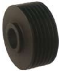
232352 Pulley Replacing: 593762 Servicing: A13VI27, A14VI27 O.D. 54.00, W. 28.50, Grooves 6, Bore 17.00
