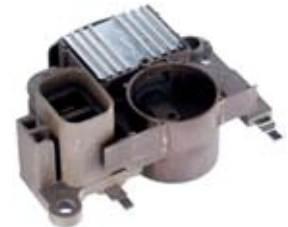
135032 Regulator Replacing: A866X21072, A866X17082, A866X17072 Servicing: A2T13977, A2T18177, A2T18277, A2T18874, A2T19677, A2T19877, A3T05274, A5T02677, A5T03477, A5T03479 14 V., V. setting 14.5, Terminal type S-L Repair Circuit: Cargo 232608.
