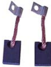
BX1572 Brush Set Replacing: 1107014142, 1107014138 12 V., L. 18.00/20.00, Th. 6.00, H. 14.00
