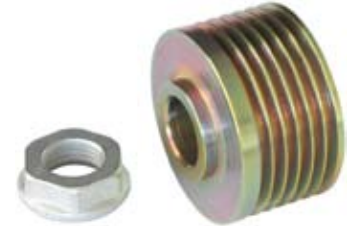
234540 Pulley Replacing: 593619 Servicing: A13VI282, SG10B023, SG8B022, SG9B064, SG9B067 O.D. 48.50, W. 31.50, Grooves 6, Bore 17.00
