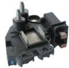
234982 Regulator Replacing: YR6620PF, 593529 Servicing: SG10B022, SG10B023, SG10B048, SG7S015, SG7S016, SG8B021, SG8B022, SG9B063, SG9B064, SG9B066, SG9B067, TG10B013 14 V., V. setting 14.6 2.5 sec. LRC.
