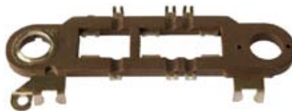
136330 Insulator For Diode Trio Servicing: A7T00191, A7T02691 O.D. 80.00, Mount. hole I.D. 9.15, Mount. holes distance 66.80,
