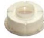
231827 Bearing Cap Servicing: A115IM., 63321678, 63321679, 63321746 O.D. 36.80/41.30, I.D. 35.00/17.80, H. 18.10
