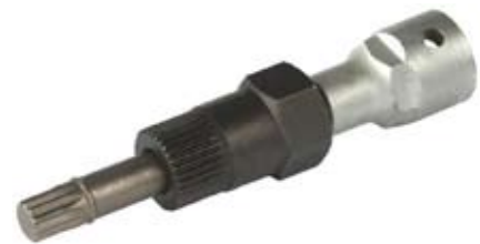
210843 Pulley Tool Tool to be used for mounting and dismounting of Free Wheel Pulley. Shaft L. 74.00mm.
