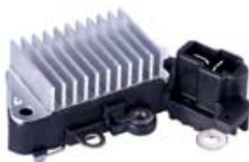
133872 Regulator Replacing: MD604751 14 V., V. setting 14.6, Terminal type IG-L Repair Circuit: Cargo 133259. The L-Terminal does not drive the choke.
