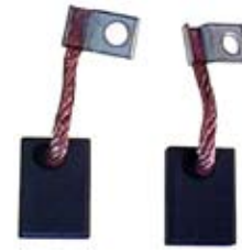
BX1692 Brush Set Replacing: 1107014144 Servicing: 0101201022, 0101203007, 0101206009, 0101206011, 0101206012, 0101206043, 0101206063, 0101206064, 0101206079, 0101206081 12 V., L. 18.00/20.00, Th. 6.00, H. 14.00
