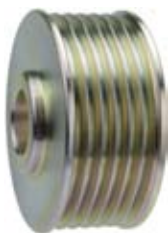
236404 Pulley O.D. 57.50, W. 30.00, Grooves 6, Bore 17.00
