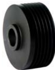
234039 Pulley Replacing: 593735 Servicing: A13VI260, A13VI261, A13VI274 O.D. 62.50, W. 31.00, Grooves 6, Bore 17.00
