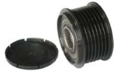
237263 Freewheel Pulley Replacing: 10493077 O.D. 56.00, W. 34.80, Grooves 7, Bore 17.00 Pulley Tool: Cargo 230843.
