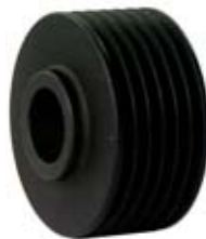
234097 Pulley Replacing: 593760 Servicing: A13VI201 O.D. 51.50, W. 29.50, Grooves 6, Bore 17.00
