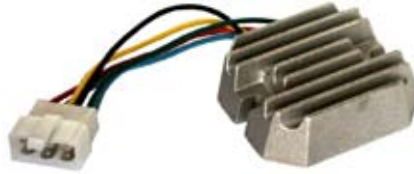
234413 Regulator/Rectifier Replacing: RS5104, RS5102 14 V. Terminals: AC(blue), -(black), AC(blue), L(green), IG(yellow), B+(red).
