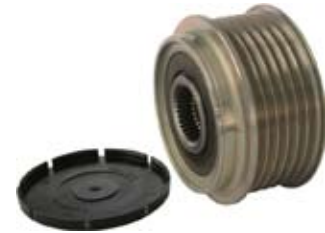
238690 Freewheel Pulley Replacing: 10511026 O.D. 59.59, W. 39.07, Grooves 6, Bore 17.00 Pulley Tool: Cargo 230843.
