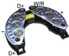
131568 Rectifier Replacing: UBB236 Diode Amp. 50, O.D. 116.00, I.D. 46.00 w/ Diode Trio. w/ Terminal W.
