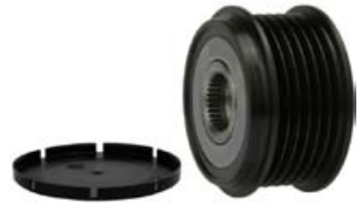
235476 Freewheel Pulley Servicing: 63321743, 63321817 O.D. 55.65, W. 35.50, Grooves 6, Bore 17.00
