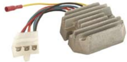
234303 Regulator/Rectifier Replacing: RS5121 14.2 V., 250 Watt, Battery sensor w/o, Insulated return No Compact tractors and industrial equipment w/ permanent magnet alternators. X: Neg. when charging. Y: Pos. when charging.
