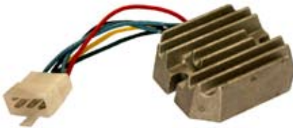
234411 Regulator/Rectifier Replacing: RS5155, RS5101 14 V. Terminals: AC(blue), B-(black), AC(blue), L(green), B+(red).
