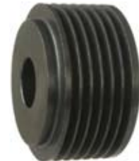
234993 Pulley Replacing: 593620 Servicing: A14VI42, SG15S016, SG15S017, SG15S021, SG15S031 O.D. 54.50, W. 29.50, Grooves 6, Bore 17.00
