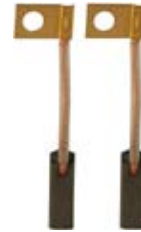
140819 Brush Set Replacing: 2660-001-10X0 Servicing: 0211-102-0012, 0211-102-0022, 0211-102-0223, 0211-102-0232, 0211-102-0412, 0211-102-2512, 0211-102-3113, 0211-102-3210 28 V., L. 18.00/20.00, Th. 6.00, H. 6.00
