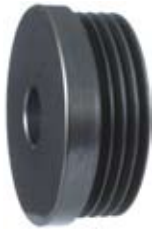
236085 Pulley Servicing: AA125R., 63320040, 63320111, 63320122, 63321136, 63321173 O.D. 60.00, W. 24.50, Grooves 4, Bore 17.00
