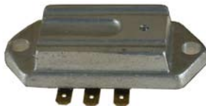
230151 Regulator/Rectifier Assy Replacing: AM106357 Diode Amp. 15, O.D. 79.90 Permanent magnet system. AC-B+-AC. Ceramic Hybrid construction. volt setting 14.2.
