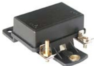
130679 Regulator Replacing: NCB211, NCB209, NCB201 14 V., V. setting 14.5 Triple phase.
