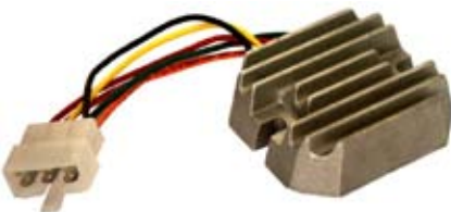
234412 Regulator/Rectifier Replacing: RS5160 14 V. 20 Amp. charging system. Terminals: B+(red), IG(yellow), B-(black), AC(orange), L(brown), AC(orange).
