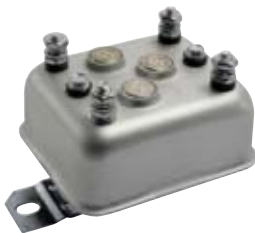
130047 Regulator Replacing: 9190215028, 0190350045, 0190350009, 0190309032, 0190215037, 0190215029, 0190215028, 0190215027 Servicing: 0010300100, 0101209016, 0101209033, 0101209039, LJ/GEH90/12/1800F, LJ/GEH90/12/1800F, LJ/GEH90/12/2300R 14 V., 90 Watt, Terminal type D+ - DF-B+, Insulated return No
