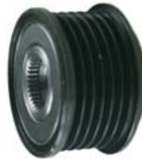
230307 Freewheel Pulley Replacing: 10453582, 10451570 O.D. 49.80, W. 35.60, Grooves 6, Bore 17.00 Pulley Tool: Cargo 210843.
